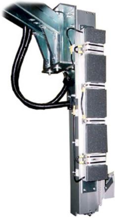
This is an option where plates weld the end of the film to the pallet.
