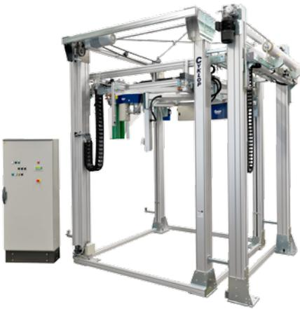
With the ITF a top film can be put on the top of the pallet to produce a dustproof or a waterproof pallet.
