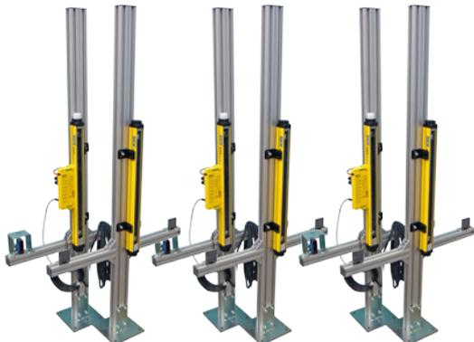
Safety application consisting of 3 sets of light beams (sender and receiver) and control unit.
