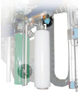
Film almost at an end is a option where the operator gets a light signal to warn him that the film roll is about to come to an end.
