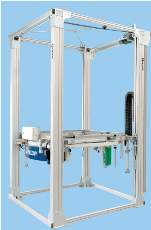
The CTR 2000 is a high performance wrapping machine, equipped with Cyklop's patented pre stretch system **POWER ECOSTRETCH** which is adjustable up to 300%.
