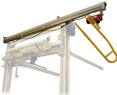
The top film loader helps to load the top film rollers into the ITF in a safe and easy way..
