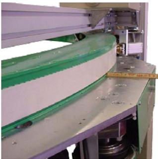
By moving the aggregate and the battery compartment, the CTR 2000 will manage +100 mm bigger pallet.
