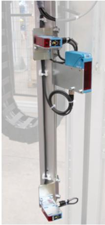
Scans the pallet to detect the height of the goods. Optimates the wrapping cycle time.
