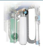
Film almost at an end is a option where the operator gets a light signal to warn him that the film roll is about to come to an end.
