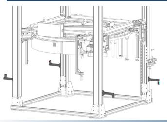
Checks that no pallet is situated on the conveyor to make sure that the ring can move freely.
