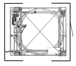
Safety fence for the CTR 2000. Also includes also a door. Total height: 2300 mm, where of the net is 2200 mm high.
