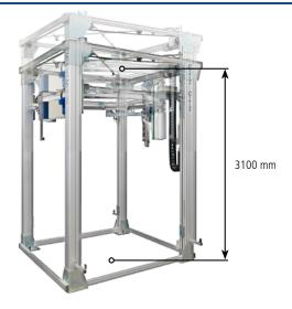
Taller CTR 2000. Used when you have high pallet loads. For pallets with height 1600 mm up to 3100 mm.
