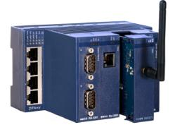
Ewon communication kit which makes it possible communicate with the machine by distance and to do changes in the program without being at the customer.
