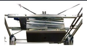
Top plate is an option consisting of a foam rubber-equipped plate that is lowered onto the goods to increase its stability.
