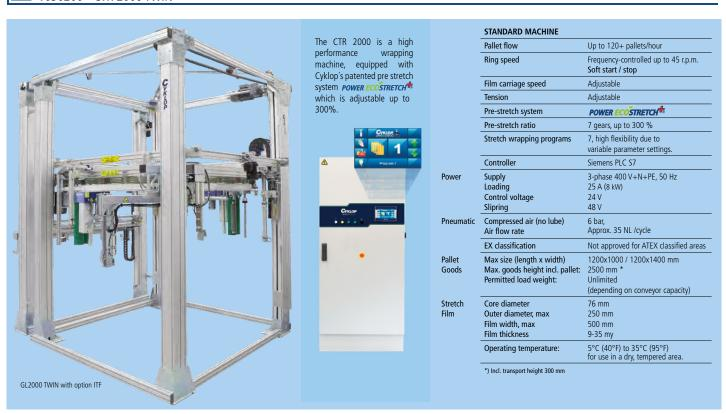
The CTR 2000 Twin is equipped with a slip ring that powers the ring and one additional pre stretch aggregate..
