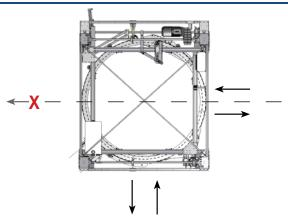
The 90° degree option is used when a straight line of transportation through the machine is not possible.
