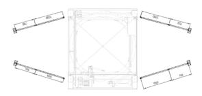
Safety fence covering the in- and/or out-feed conveyors.
