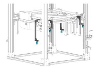
When the ring rotates the photocell works like format control and stops the machine if the pallet is inside the area where the ring moves.
